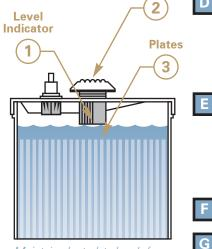
Maintain electrolyte levels from at least 1/2-inch (13 mm) above plates to 1/4-inch (6 mm) below level indicator.
